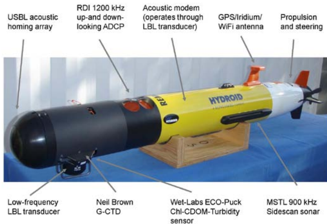
Fig. 2. The REMUS-100 AUV as delivered. The location of principal systems and sensors is shown.
