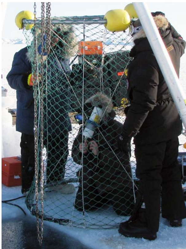
Fig. 4. Photo of the AUV capture net being prepared for deployment. Note the USBL homing beacon being suspended inside the net.
